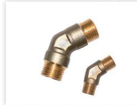
**Screw-in fitting 45°, inch thread, symmetric, brass, 60° cone**
